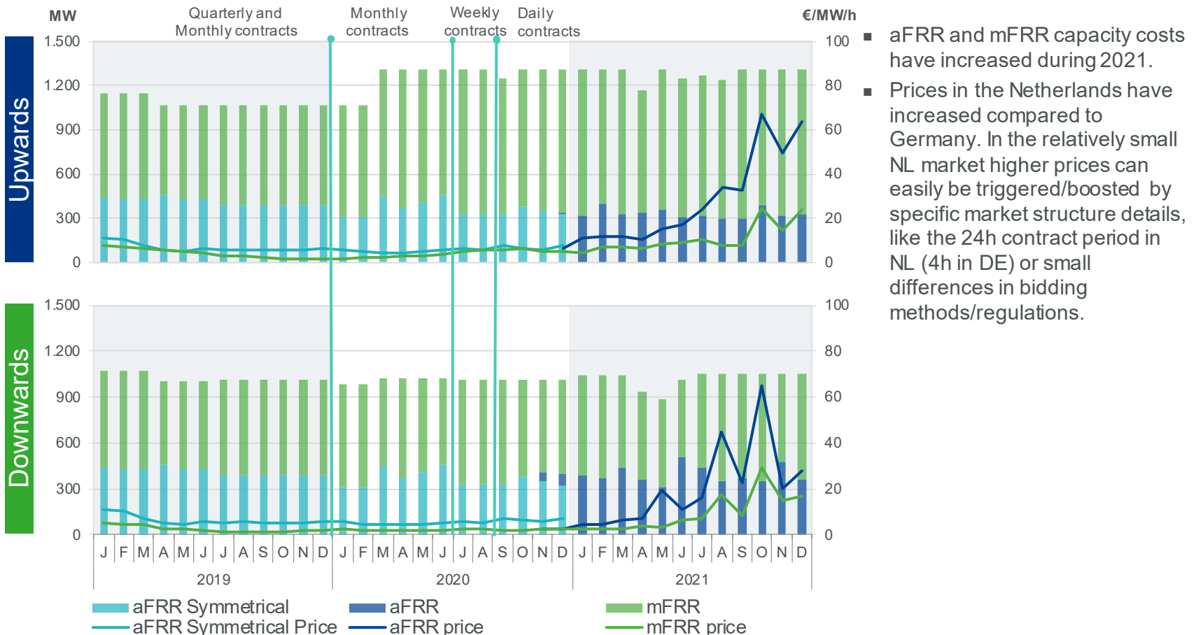
Contracted automatic Frequency Restoration Reserve (aFRR) and manual Frequency Restoration Reserve directly activated (mFRRda) Capacity Volumes and Prices in the Netherlands
