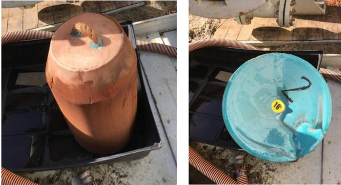
Figure 11. Foam pig, on the left front side and on the right back side.
