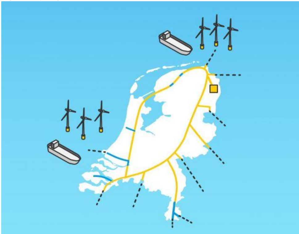
Figure 1. Hydrogen backbone in the Netherlands (Hynetwork Services).
