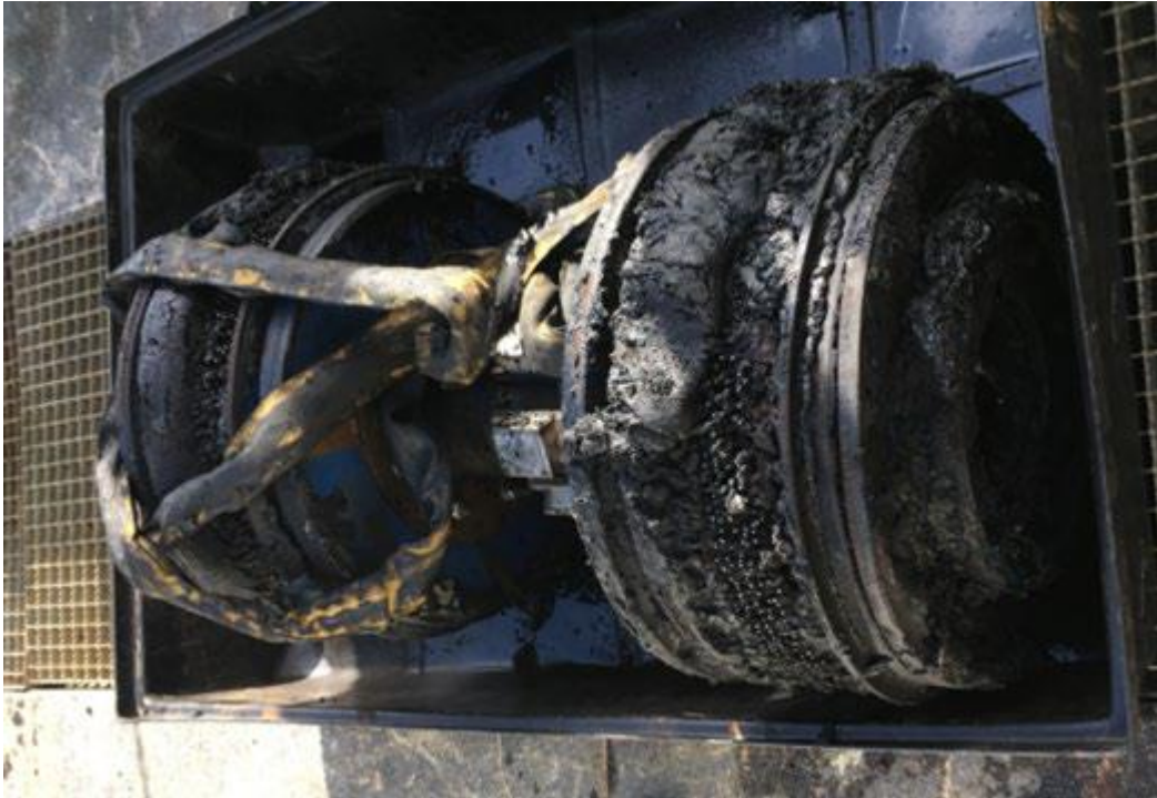
Figure 14. Dirty tool after pigging a natural gas pipeline.
